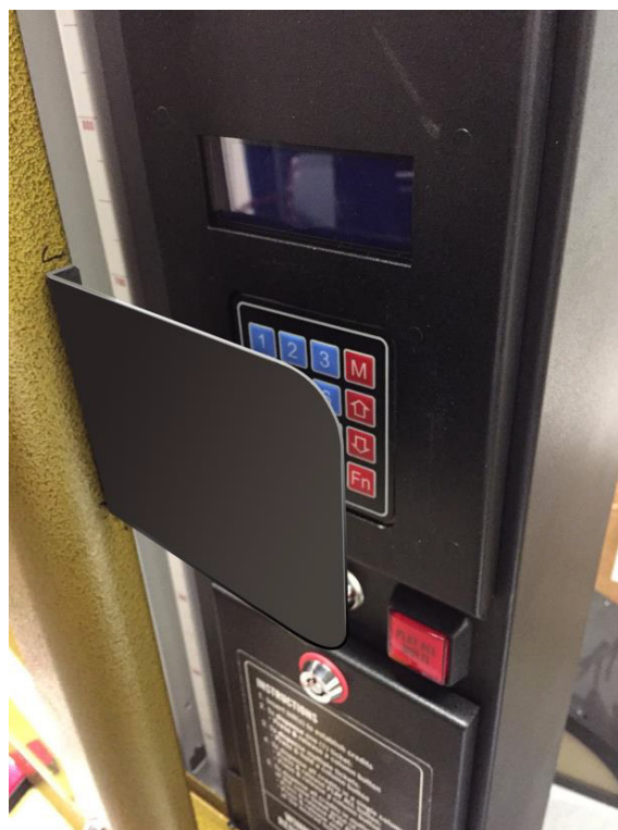
Opening of the main door for service exposes the keypad, enabling password entry.
